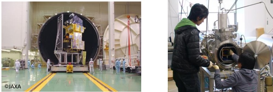
Figure 17 Thermal vacuum test of large satellites (left) and thermal vacuum test of lean satellite (right)
