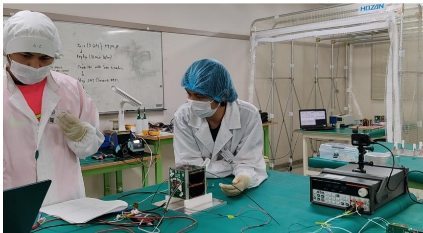
Figure 10 State of the System Functional Test (The satellite is placed on the test jig)
