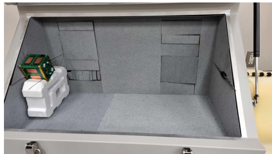
Figure 6 Receiver Sensitivity Test in the Shielded Box
