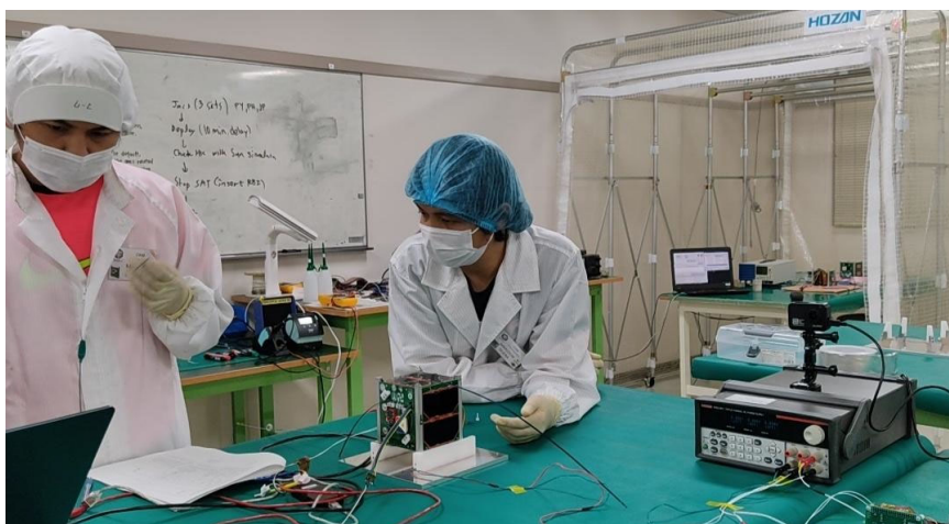
Figure 5 State of the System Functional Test (The satellite is placed on the test jig)
